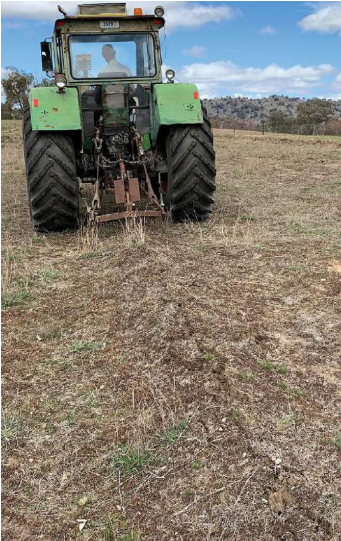
Fig 2.15: The first rip using a tractor-based single tyne.
