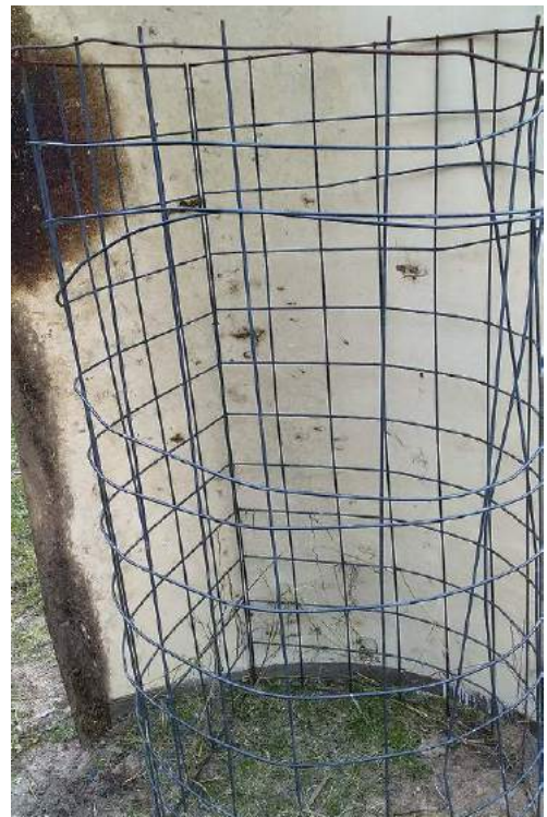
Fig 7.17 (right): Cheap 3 mm lightweight imported mesh which has been badly damaged by cattle reaching in to eat the top off a young paddock tree. Photo by Keith Hyde.
