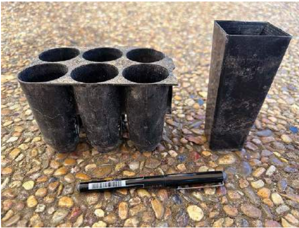
Fig 4.6: Six 85 mm high Hiko pots cut from a larger Hiko tray of 40 pots and a 120 mm high forestry pot.
